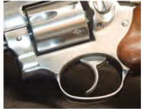
† The fit and finish show no signs of damage or uneven gaps. The trigger is centered in the opening.
