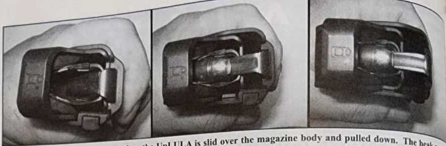
Above: Left - To load the magazine, the UpLULA is slid over the magazine body and pulled down. The beak pushes downward on the magazine follower. Center - The next step is the round is slid on top of the beak into the magazine. Right - Now the lever is released and the beak slides out from underneath the cartridge fully seating it inside the magazine. To insert additional cartridges the same process is repeated with the only difference being the beak pushes down on the top cartridge instead of the magazine follower.
